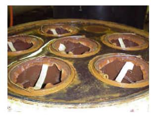
After 15 days of treatment, scale was soft and easily removed. Bag filter is required to be changed every 5 to 6 days.
