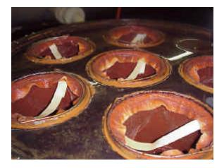
After 45 days of treatment, scale was entirely removed and no new scale was formed. Bag filter is only required to be changed every 10 to 11 days.
