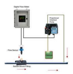
Typical injection system treats water proportional to flow in the main water line.
