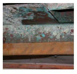
Initial hard deposites on duct surfaces forms within a few days.
