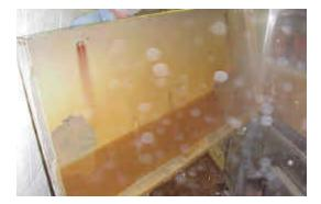
Initial mineral scale is hard and deposits on the panel of the pasteurizer. Picture shown before Oxcide treatment.
